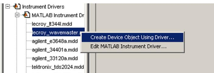
Figure 3. Creating an instrument object from a driver.
