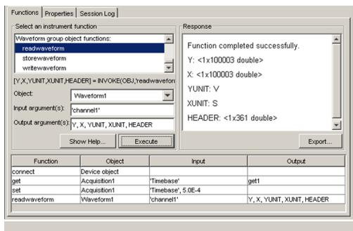
Figure 5. Invoking `readwaveform` of an instrument object.
