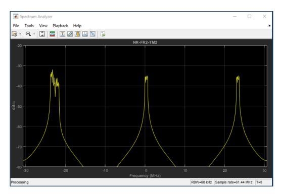
Figure 2. Spectrum of NR-FR2-TM2 waveform with 50 MHz bandwidth and 60 kHz subcarrier spacing.
