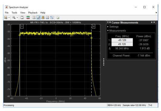
Figure 4. Spectrum of NR-FR1-TM3.1a waveform with 100 MHz bandwidth and 30 kHz subcarrier spacing.
