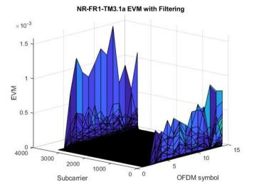
Figure 9. EVM of the filtered NR-FR1-TM3.1a waveform for each resource element in the last slot.
