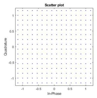
Figure 8. 256QAM constellation recovered in the receiver.
