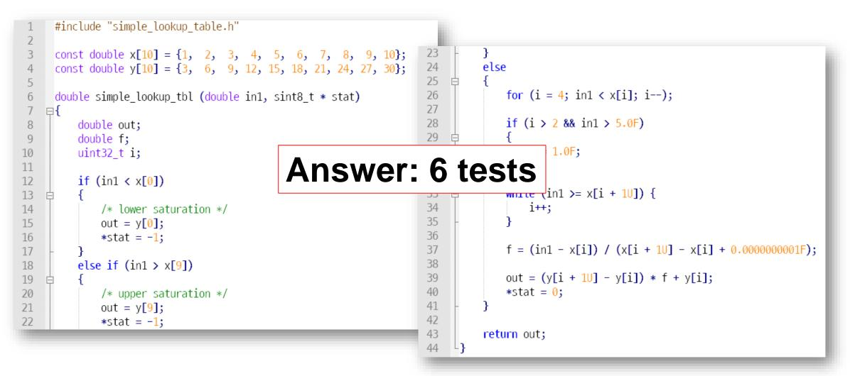
Automatically-generated test for input = 5.9566, 1.9184, -5.4067, 9.8142, 11, 4
