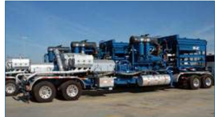
Truck with positive displacement pump.
