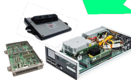
Embedded Controller Hardware
