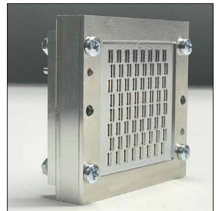
▲ Fig. 7 The single polarization Gapwaves antenna is an 8 \times 8 slot array configured as 4-slot subarrays in eight columns and two rows.
